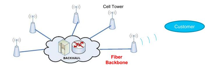
The below "two-fiber" example shows a cell tower fiber backbone outfitted with a common 8-channel CWDM filter pair to increase data-carrying capacity
